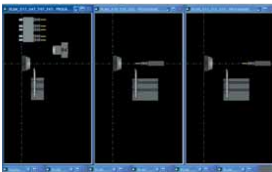
Graphic machining simulation and assistant graphic showing programming programmed contour.
