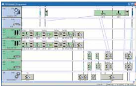
Display of the Gant chart program with exact calculation of the cycle time for each operation and the part.
